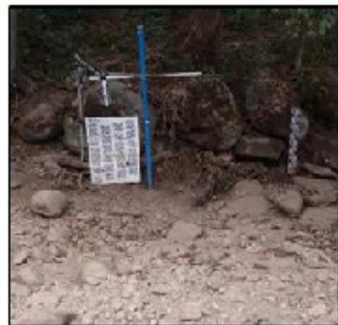
W1 tributary in summer 2020, left QR-code plate + camera, right: Odyssey water level logger
